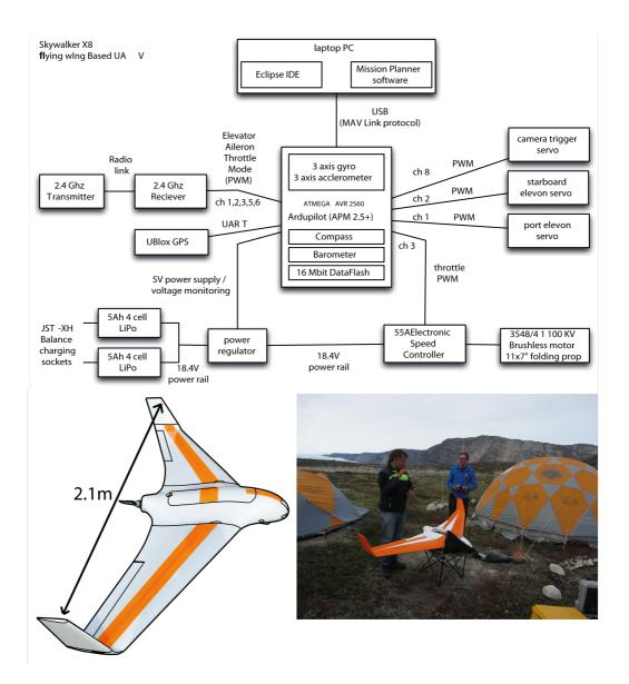
**Figure 2.** Flowchart of the control set up and picture of the UAV at base camp with the 'relative novices'.
