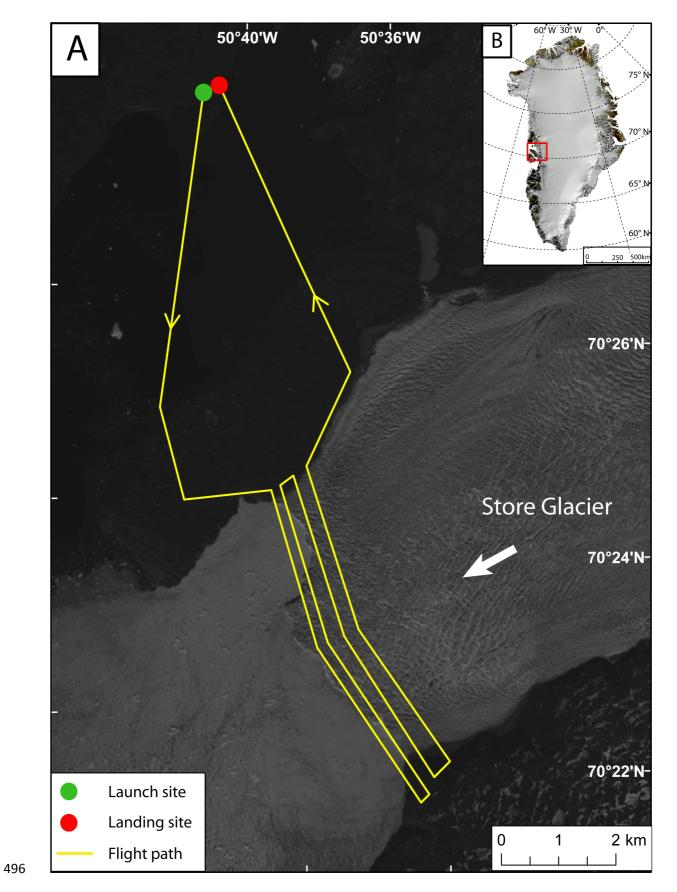
**Figure 1.** (A) The planned UAV mission over Store Glacier. The background map is a Landsat 8 panchromatic image from 12 June 2013. The green and red dots show the launching and landing sites and the yellow line shows the planned UAV mission. (B) Location of Store Glacier in the Uummannaq Region, West Greenland on a MODIS mosaic image of Greenland (Kargel et al., 2012).
