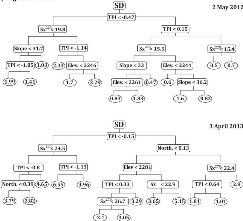
**Fig. 7.** Binary regression tree obtained for 2 May 2012 (top) and 3 April 2013 (bottom). The final nodes (with ellipses) show the predicted SD in the zone having the specified terrain characteristics. At each branch point, one topographic variable is considered; if the value is less than the specified value, the left branch is selected, but if it is equal to or greater than the specified value, the right branch is selected.
