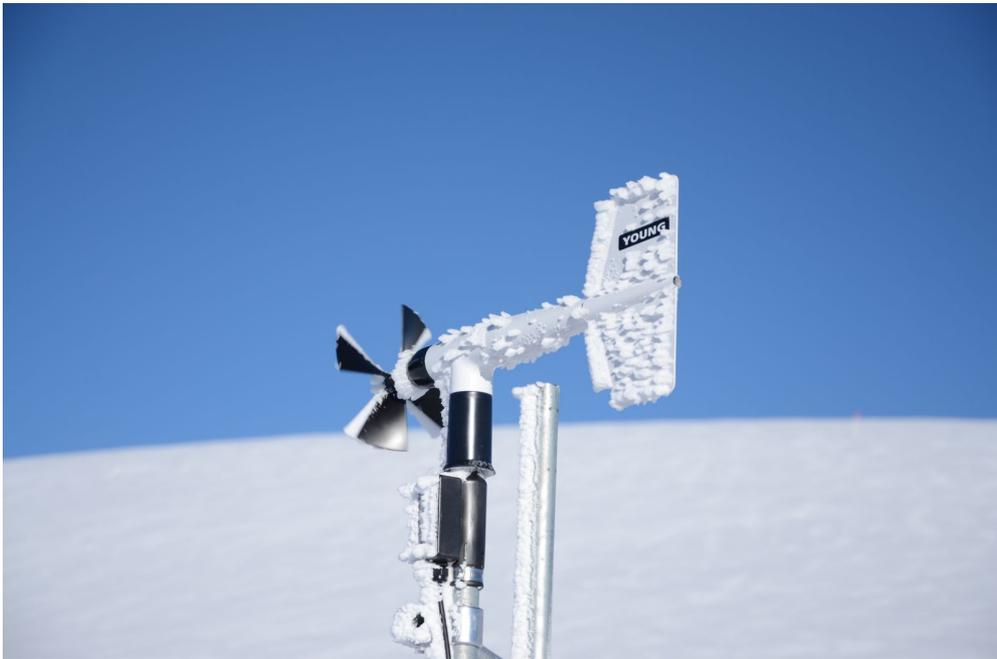
*Figure 4 – Picture of the anemometer showing the presence of hoar on October 4<sup>th</sup>.*
