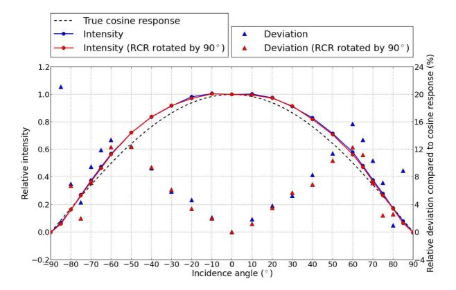
The plot shows the angular response of our RCR at 500 nm, for incidence angles ranging from -90° to 90°. Relative intensities normalized by I(0°) are represented by blue circles and compared to the true cosine response (dashed black line). Blue triangles represent absolute values of cosine collector fractional errors ( $\epsilon_{\lambda}$ ) as a function of the zenith angle of the incident light (deviation of the measured response from a true cosine response), computed as follows:
