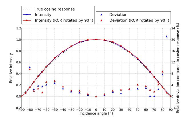
The spectral albedo has been then corrected taking into account this cosine collector deviation from a true cosine response (Equ. 10 of the revised manuscript):
