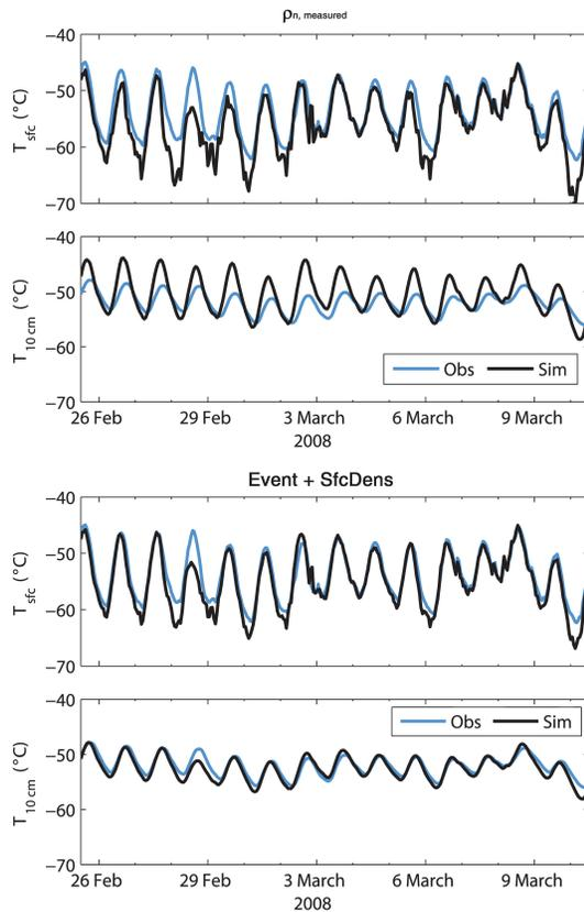
**Fig. 6.** Observed (Obs) and simulated (Sim) snow surface temperature  $T_{\text{sfc}}$  and snow temperature  $T_{10\text{cm}}$  at 10 cm depth. The two upper panels relate to the simulation “ $\rho_{n, \text{measured}}$ ”, the two lower ones to the event-driven simulation “Event + SfcDens”, that is, with additional wind densification at the surface.
