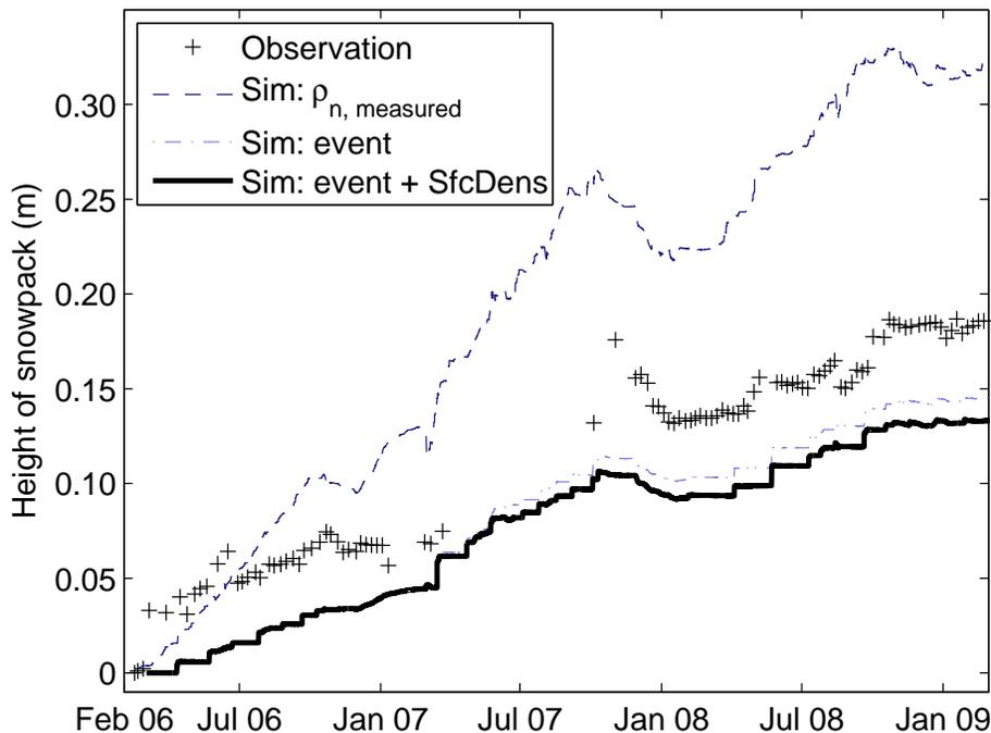
**Fig. 5.** Height of snow (cm) relative to the snow layer which was at the surface on 15 February 2006. Stake measurements are indicated by crosses, and lines represent results from SNOWPACK simulations using either the measured density of new snow as input (“ $\rho_{n, \text{measured}}$ ”), or the event-driven mechanism without (“Event”) or with additional densification due to wind at the surface (“Event + SfcDens”).
