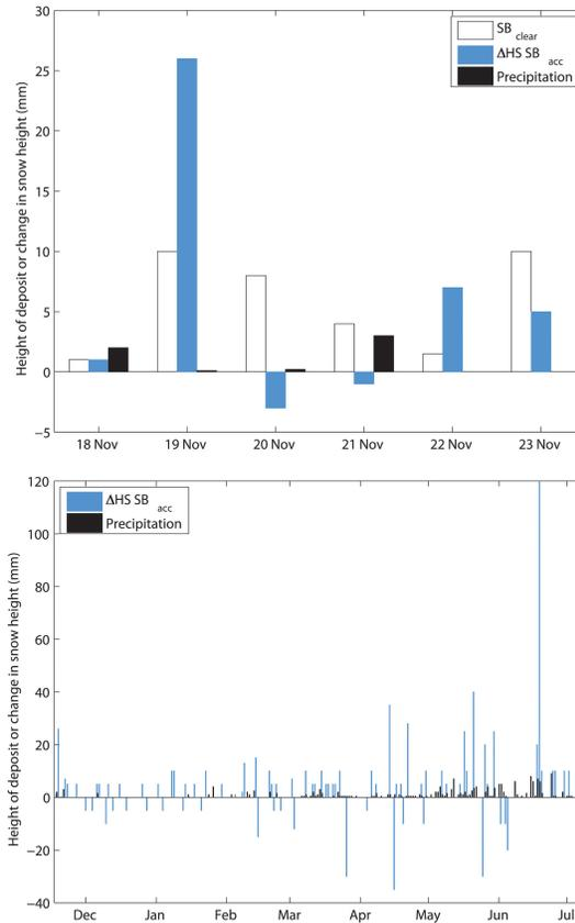
**Fig. 4.** Height of deposits (mm) measured daily either on a table 1 m above the surface (Precipitation) or at the surface on a daily cleared snow board ( $SB_{clear}$ ), and change of snow height  $\Delta HS$  over an untouched snow board ( $SB_{acc}$ ). Top panel: 18–23 November 2008; Bottom panel: 18 November 2008 through 3 July 2009, board  $SB_{clear}$  not shown.
