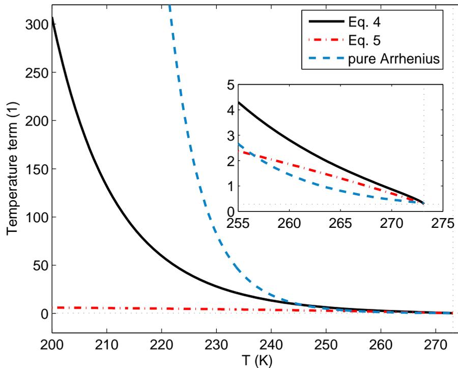
**Fig. 3.** Temperature term of the viscosity according to Eqs. (4) and (5).
