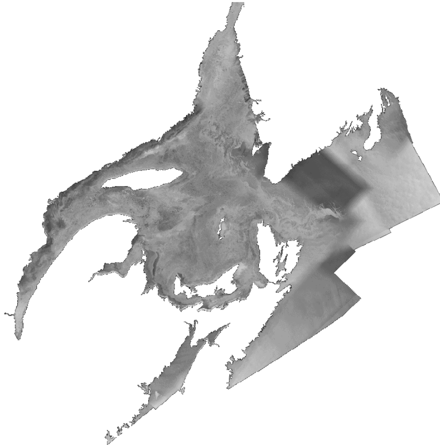
Fig. 5. An example of a SAR mosaic (based on RADARSAT-2 data, © MDA), on 5 March 2009, the boundaries between SAR frames have been smoothed in the mosaic.
