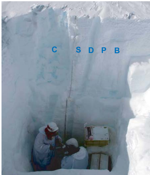
Fig. 3. A picture of the pit wall at DF on 10 December, 2007. Two scientists are collecting firn samples in the pit. Letters indicate positions of measurements or sampling for different purposes. P is for the permittivity measurements with the snow fork. D is for density measurements using a box sampler. S is for observing stratigraphy and temperature measurements. B is for sampling firn blocks for analyses of physical properties. C is for sampling snow for chemistry purposes.
