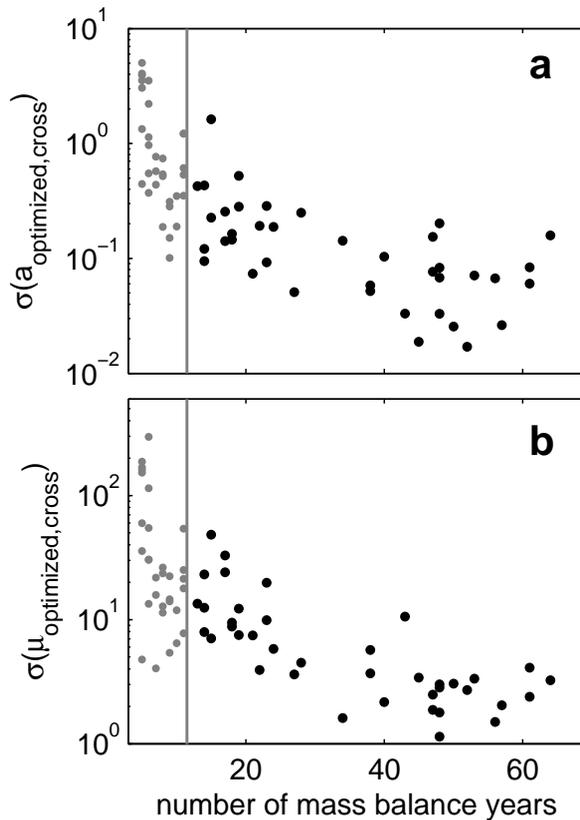
**Fig. 3.** Standard deviation of  $a_{k,\text{cross}}$  **(a)** and  $\mu_{k,\text{cross}}$  **(b)** as a function of the number of mass balance measurements. Black dots are the values of glaciers accepted into the final set, gray dots are those of the glaciers rejected from the final set. The gray vertical line indicates the minimum number of mass balance measurements necessary to obtain robust results for  $a_{\text{optimized}}$  and  $\mu_{\text{optimized}}$ .
