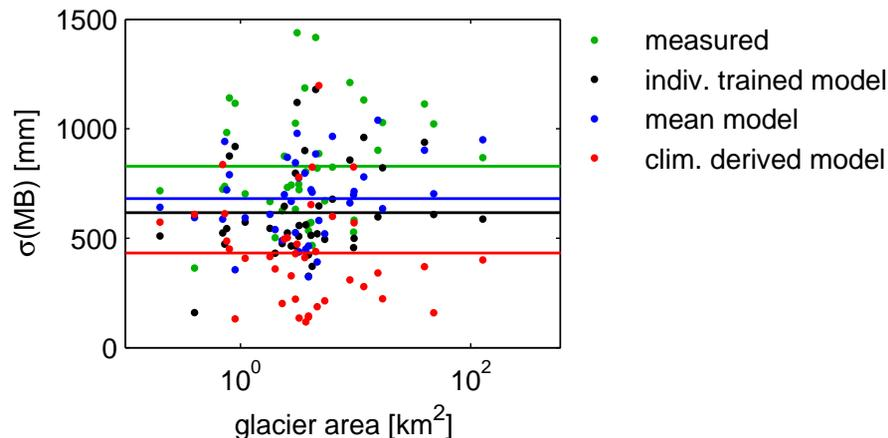
**Fig. 5.** Standard deviation of the annual mass balance plotted against the area of the glaciers. Green dots show  $MB_{\text{measured}}$ , black dots show the values of the individually trained model, blue dots show the results of the mean model, and red dots show the results of the climatologically derived model. Horizontal lines show the respective means.
