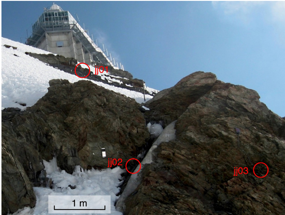
Fig. 3. Close-up of sensors in densely fractured rock at the south side of Sphinx, Jungfrauoch. The picture is taken in April 2007 after a periode with intense irradiation.
