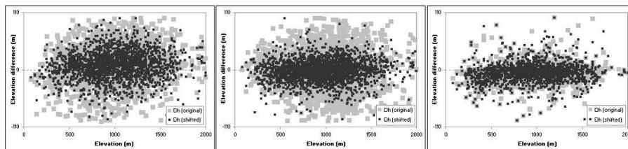
**Fig. 6.** Comparison of the original and shifted data for (from the left to the right) the 1975 DEM, SRTM and SPOT 5 DEM of 2005.
