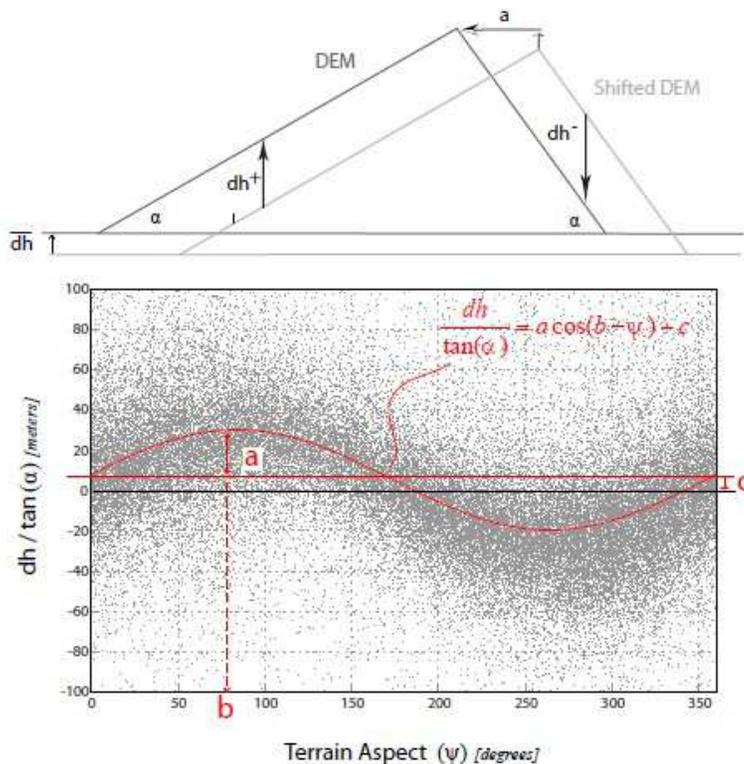
**Fig. 4.** Published by Nuth and Kääb (2011): Top: 2-D scheme of elevation differences induced by a DEM shift. Bottom: The scatter of elevation differences between 2 DEMs showing the relationship between the vertical deviations normalized by the slope tangent (y-axis) and terrain aspect (x-axis).
