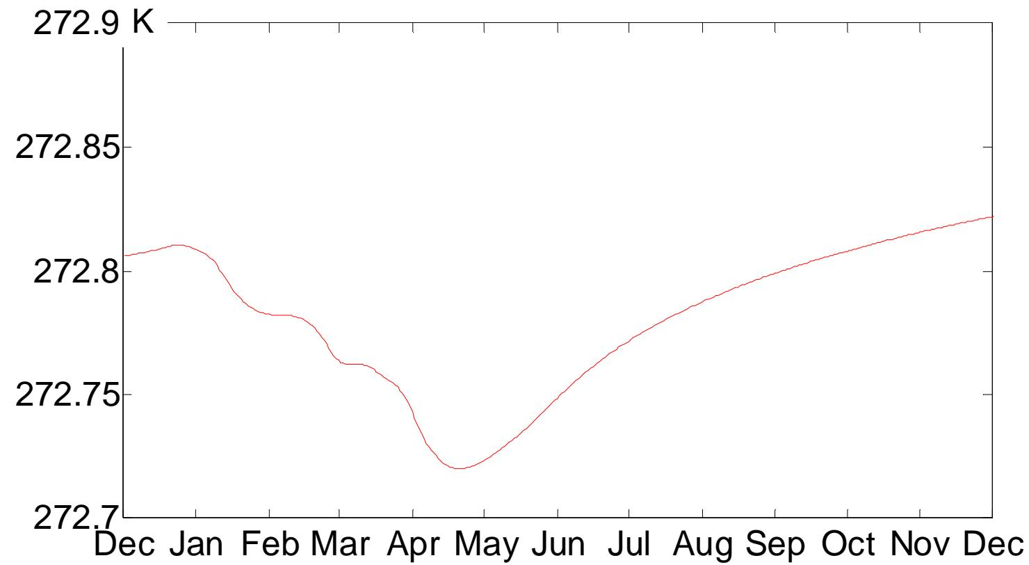
Fig.2: Temperature at the ice-rock interface
