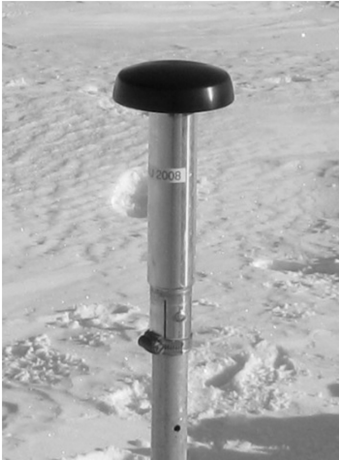
Fig. 1. GPS unit attached to a mass-balance stake.
