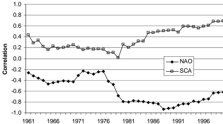
**Fig. 6.** Running 21-year correlations between the NAO and SCA modes of NH winter (JFM) circulation and NH March SCE. Correlations exceeding 0.4 are nominally significant at a 0.05 level assuming data series are not autocorrelated.
