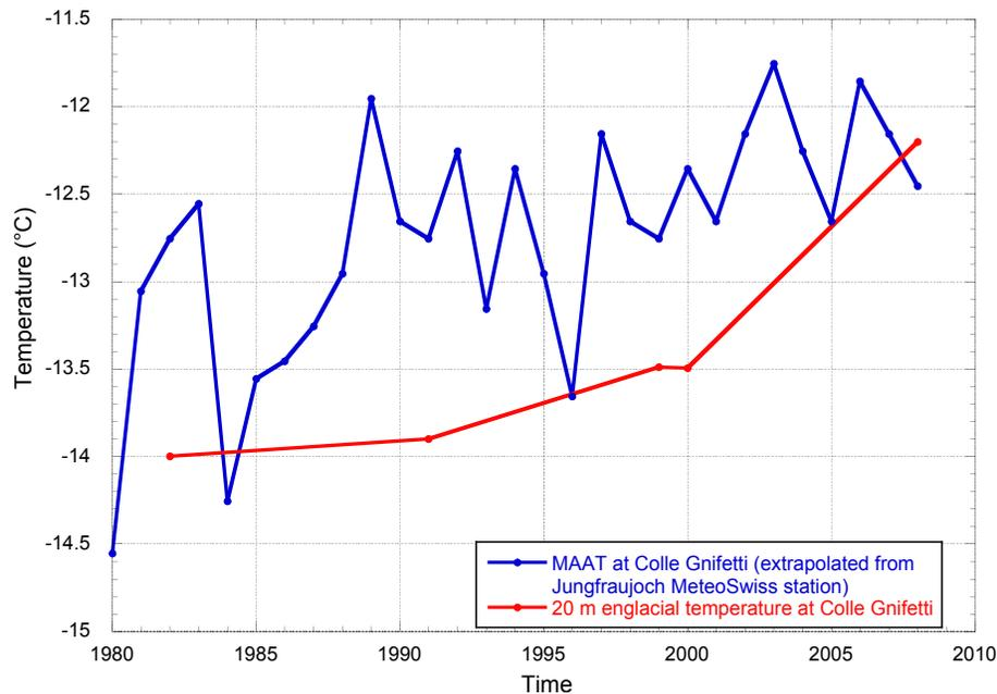
**Fig. 10.** Measured annual air temperatures at Jungfrauoch extrapolated with a lapse rate of  $6.5^{\circ}\text{C km}^{-1}$  to the altitude of Colle Gnifetti and firn temperatures at a 20 m depth at Colle Gnifetti.
