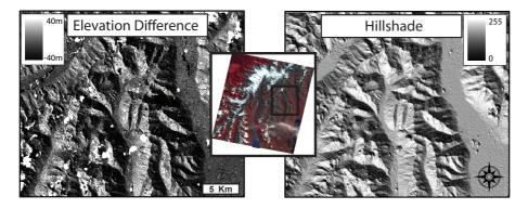
**Fig. 1.** The elevation differences before shifting (left) between ASTER DEMs in 2006 and 2002 from New Zealand (described in Sect. 5.3 and shown in Fig. 7) are remarkably similar to the hillshade of the DEMs (right). The location of the subsetted region is depicted in the 2006 ASTER image (center).
