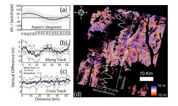
**Fig. 7.** (a), (b) and (c) show the first three corrections applied between two ASTER SilcAst DEMs from 2006 and 2002. (d) shows the resulting elevation differences with a plot of the mean elevation differences along track. The linear cross-track features that run along track seem to have an amplitude of 1-2m in the vertical direction. These fluctuations are thought to be induced by unrecorded pitch variations of the satellite, *jitter*.
