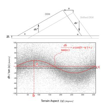
**Fig. 2.** Top: 2-dimensional scheme of elevation differences induced by a DEM shift. Bottom: The scatter of elevation differences between 2 DEMs showing the relationship between the vertical deviations normalized by the slope tangent (y-axis) and terrain aspect (x-axis). The example is the DEM differences between the 2002 and 2003 DEM used in Case Study 1 (Sect. 5). The equation for the solved sinusoidal curve fit is shown along with the three unknown solution parameters, *a*, *b* and *c*.
