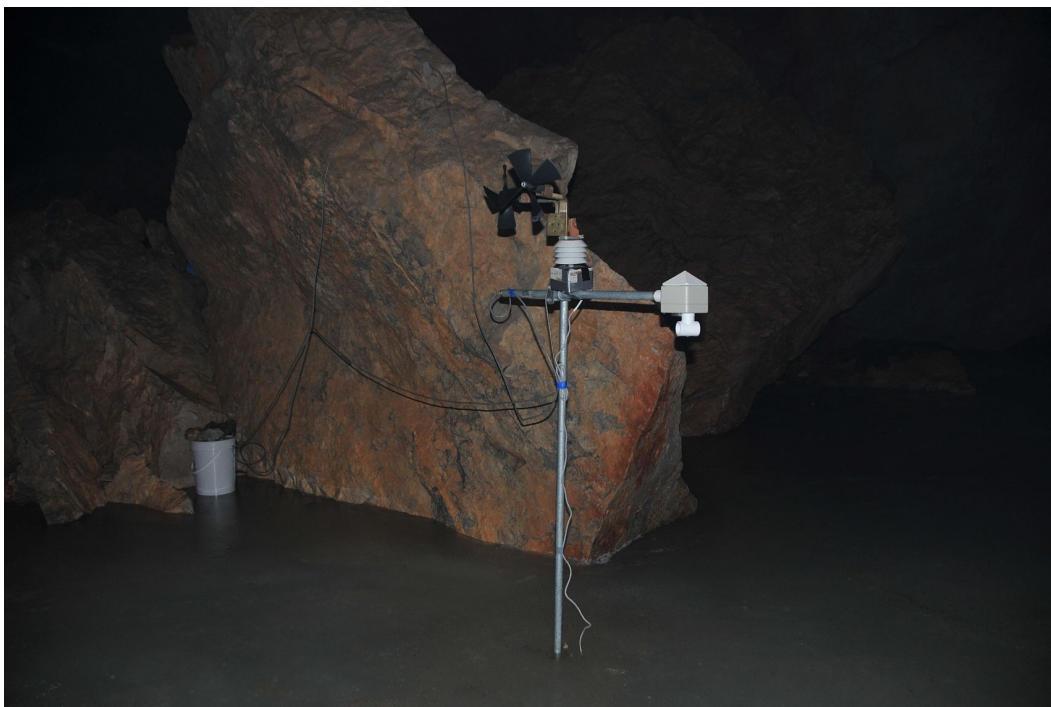
Fig. 3. The automatic weather station AWS in the central part of Eisriesenwelt at site Odinsaal (see Fig. 1 for location of the AWS).
