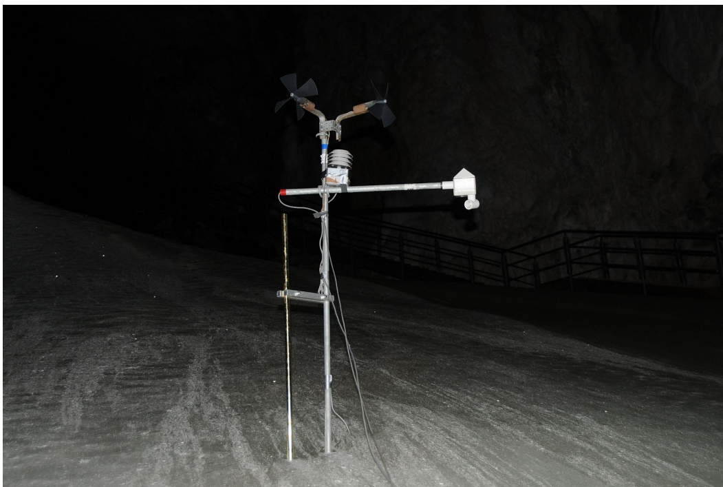
Fig. 2. The automatic weather station AWS close to the cave entrance at site Posselthalle (see Fig. 1 for location of the AWS).
