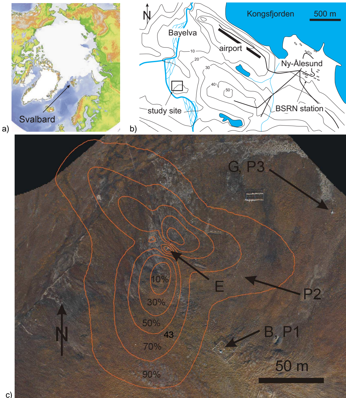
Fig. 1. a) Map of the Arctic. b) Location of the study site and the BSRN site; thick black lines: roads; contour lines in meters above sea level. c) Orthorectified aerial photo with all installations (E: eddy covariance system; B: Bayelva climate station; G: gradient tower; P1, P2, P3: temperature profile measurements). The average footprint of the eddy covariance system from 1 July to 30 September 2008 is shown, with the percentages of the total flux originating within the respective contours.
