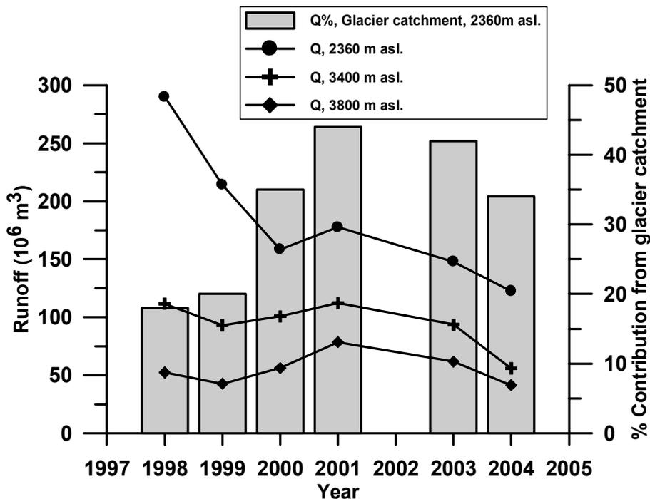
**Fig. 6.** Stream discharge variations observed at three elevations of the Din Gad catchment and corresponding variations in the contribution from the glacier catchment at 2360 m a.s.l. during the study period.
