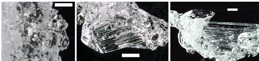
Fig. 3. Photomicrographs illustrating the formation of depth hoar from the melt-freeze crust studied in Alaska. Samples are from (left to right) 11 November 2003, 27 January 2004 and 12 February 2004. Scale bars: 1 mm.
