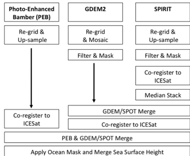
**Figure 3.** Schematic of the approach used to produce the GIMP DEM from the three source data sets.
