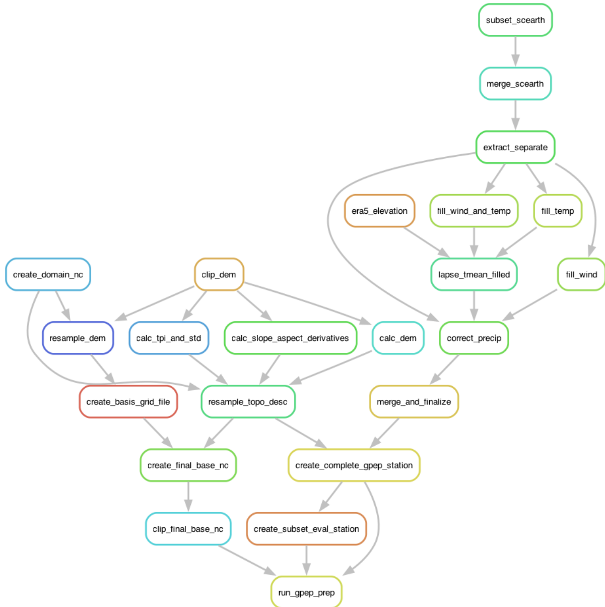
Figure S1: Autogenerated Snakemake workflow image example depicting static input data generation for GPEP. The workflow orchestrates a series of preprocessing steps to prepare gridded and meteorological station input data.
