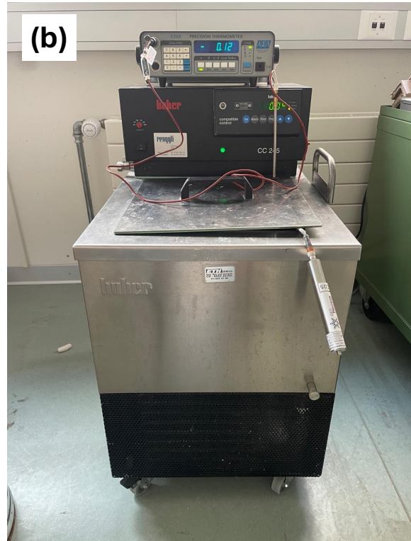
Figure S5. Temperature-controlled baths used for calibrating thermistor sensors prior to field deployment. (a) Ice bath used to determine 0 °C offsets for Tinytag thermistors. (b) Alcohol bath (Huber CC245 WL) and high-precision thermometer (ISOTECH F250) used to determine 0 °C offsets for Geoprecision thermistors.
