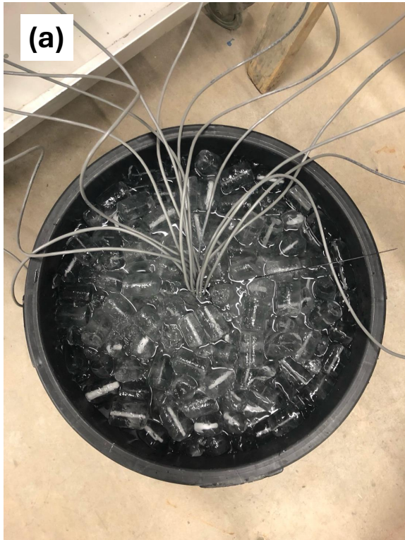
Figure S5. Temperature-controlled baths used for calibrating thermistor sensors prior to field deployment. (a) Ice bath used to determine 0 °C offsets for Tinytag thermistors. (b) Alcohol bath (Huber CC245 WL) and high-precision thermometer (ISOTECH F250) used to determine 0 °C offsets for Geoprecision thermistors.
