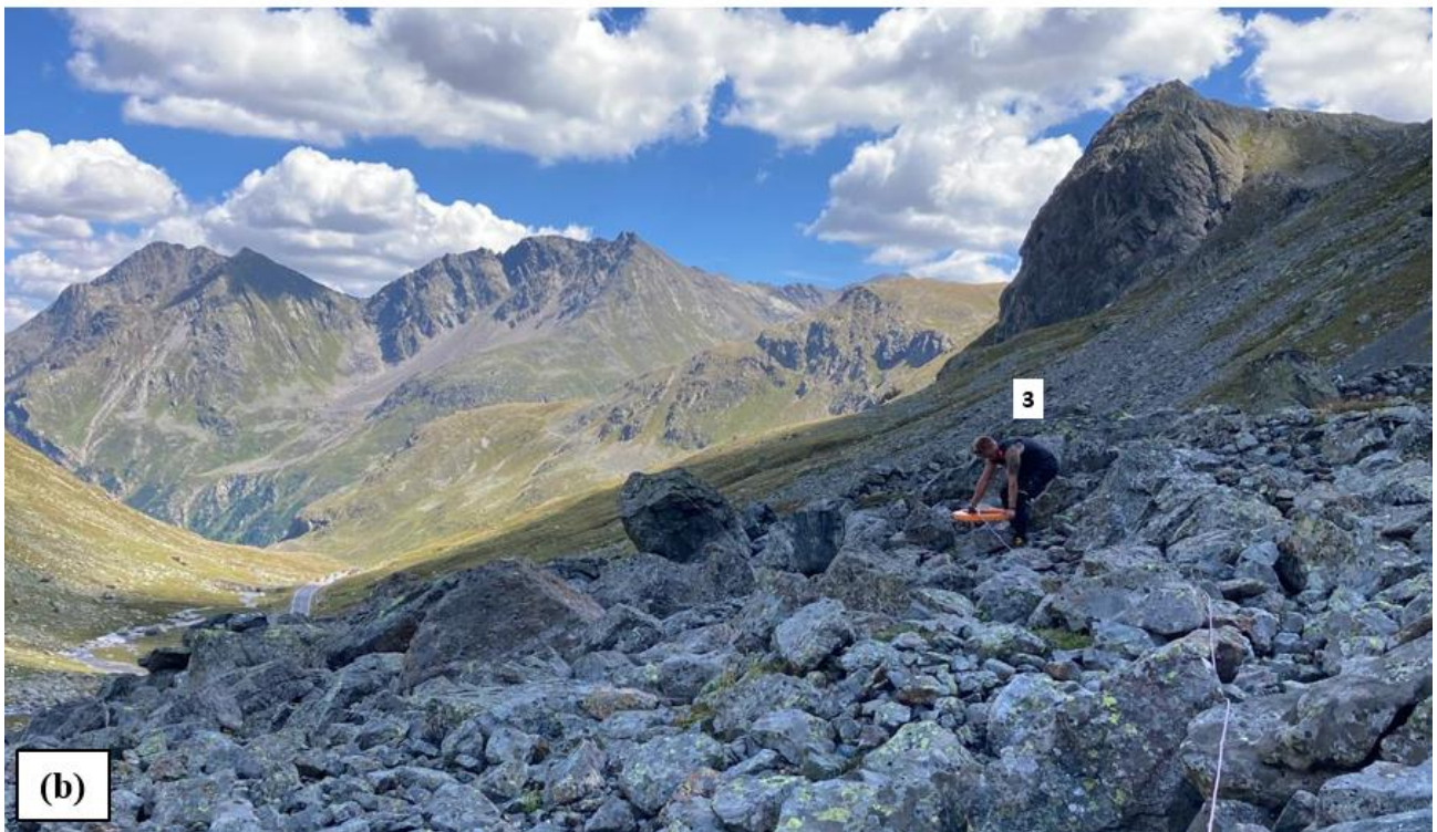
1 2 Figure S1. Photographs of FDEM data acquisition using the separable dual-coil CMD-DUO system (GF Instruments) on the Flüela 3 Pass rock glacier (Fig. 1a), in HCP configuration with a coil separation of 40 m. In panel (a), operator 1 holds the data logger (with 4 integrated GPS) and operator 2 holds the transmitting antenna; in panel (b), operator 3 holds the receiving antenna. The thin purple 5 cable connecting the two antennas is visible. Note that the blocky, rough, and irregular surface of the rock glacier makes it 6 challenging to optimally positioning the antennas (orientation) and the connecting cable (distance), which likely affect the 7 measurement quality.
