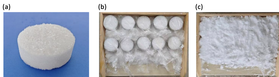
Figure 1. Sample preparation process (a, compacted specimen; b, samples covered with membranes; c, sprinkling snowflakes).
