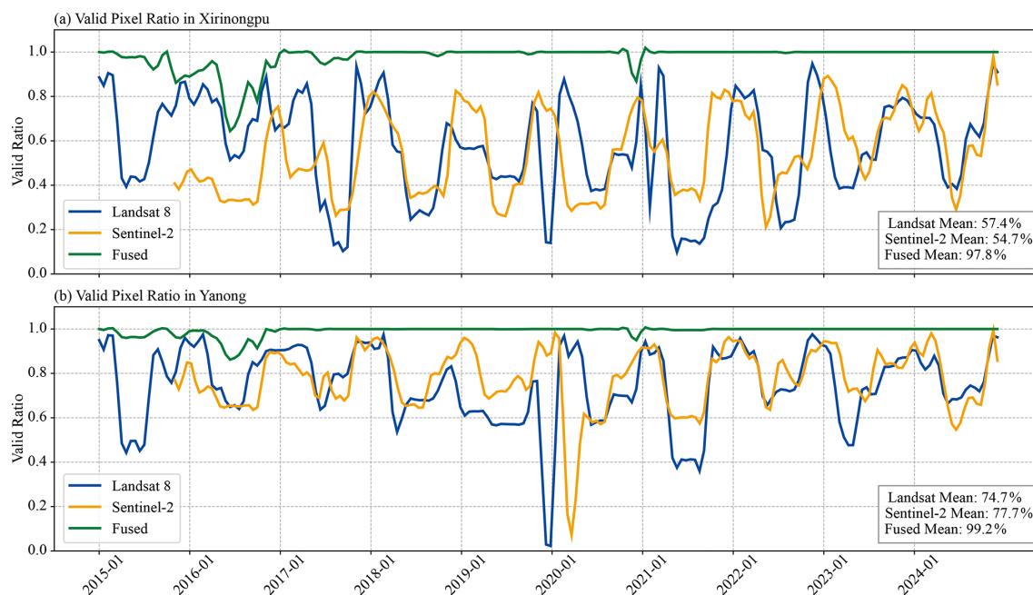
Figure 3. (a) Xirinongpu Glacier; (b) Yanong Glacier – proportion of valid pixels before and after fusion.
