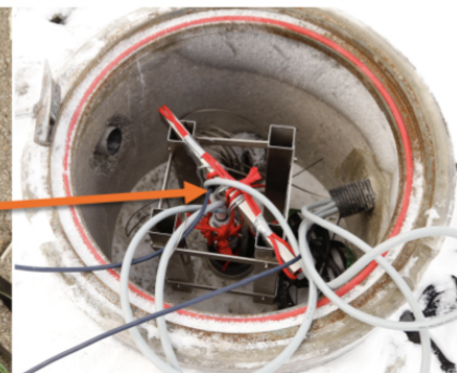
Figure 2. The installation of the 2015 borehole in Murtèl rock glacier. Sketch of the top-down cross-section of the borehole (top-left). Photo of the drilling of the 2015 borehole (top-right). Configuration of thermistor-inclinometer bundle inserted in the borehole with its top concrete chamber (bottom). Photos by Alexander Bast.
