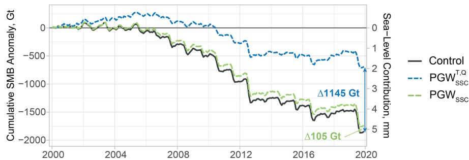
Figure 4. Temporal evolution of the SMB under contrasting thermodynamic background conditions. Shown are the cumulative SMB anomaly time series for the control (gray), \text{PGW}_{\text{SSC}}^{T,Q} (blue dashed), and \text{PGW}_{\text{SSC}} (green dashed) simulations. Anomalies calculated with respect to the 1980–1989 reference period. Left axis shows cumulative SMB anomaly; right axis shows the equivalent sea-level contribution. Annotations detail the difference in the final cumulative SMB between each of the PGW simulations and the control.
