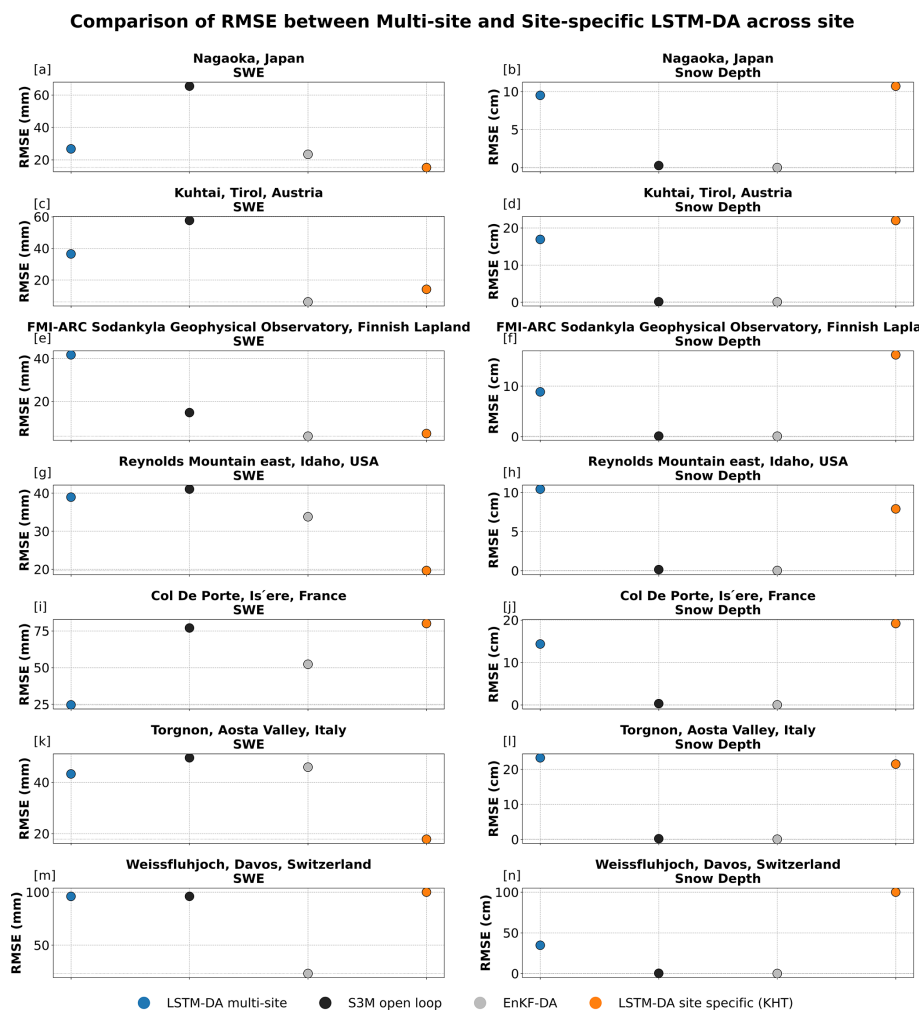
Figure 9. Comparison of RMSE for snow water equivalent (SWE, left column) and snow depth (right column) across multiple sites and methods. Results are shown for LSTM-DA multisite (blue), S3M open loop (black), EnKF-DA (grey), and LSTM-DA site-specific (orange).
