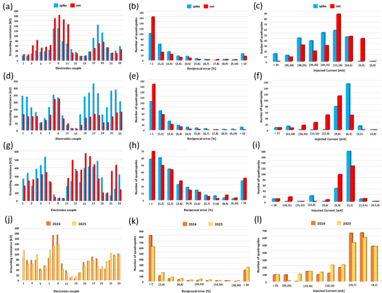
Figure 2. Histograms (a), (d), and (g) compare grounding resistances [kΩ] recorded at the Marocche di Drò, Sadole, and Flüela test sites, respectively, using traditional stainless-steel spike electrodes with sponges (blue) and the proposed stainless-steel net electrodes (red). Panels (b), (e), and (h) show the corresponding reciprocal error [%] of the quadrupoles for the same sites and electrode types, while (c), (f), and (i) present the injected electric currents [mA]. All electrodes were moistened with the same amount of saltwater and placed at comparable positions between surface boulders (see Fig. 1b–c). Panels (j), (k), and (l) illustrate the contact resistances (first 24 electrodes, as in panel a), reciprocal error, and injected current for datasets acquired at the Sadole site in June 2024 (orange) and June 2025 (yellow) along the permanent ERT monitoring line using the stainless-steel net electrodes.
