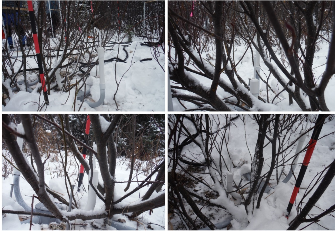
Figure S1. Photographs of the S325 and S485 sensors during installation on December 2 nd 2020. The S325 sensor is at the center of the shrub while the S485 sensor is near its edge. The nails were hammered into the ground shortly afterwards to ensure they would not perturb radiation transfer. The snow visible here melted entirely on December 25 th (Figure 6). The color stripes on the snow stake are 10 cm high.
