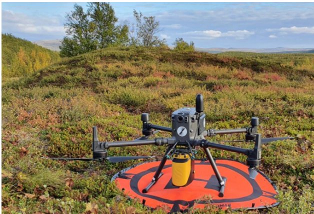
Figure 3. DJI Matrice 300 RTK equipped with the YellowScan Mapper+ in front of the Ridge palsa.
