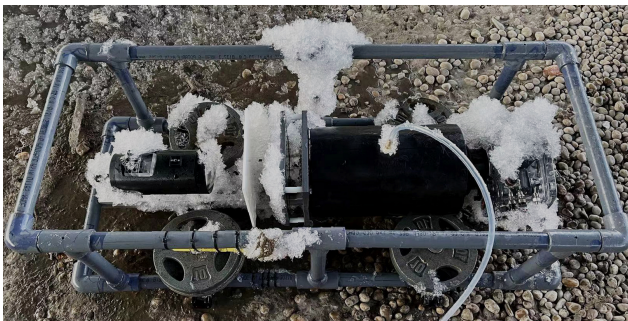
Figure 3. An image showing the ice accumulation on the FrazilCam system.
