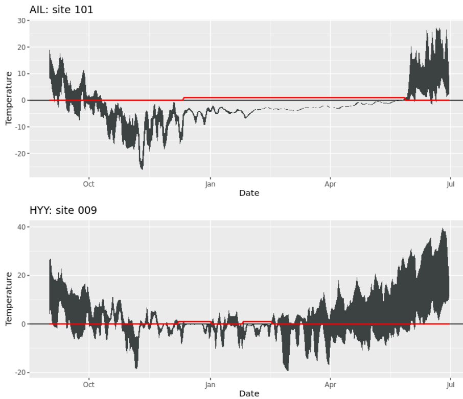
Figure A1. Examples of detecting snow cover duration from the temperature time series. The dark grey colour shows daily maximum and minimum values of near-surface air temperatures (+15 cm), and the red line indicates when the algorithm detects snow cover (0 for no snow cover, 1 for snow cover).
