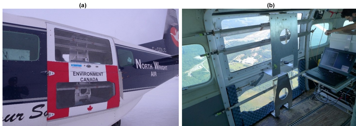
Figure 1. UMass Ku-band radar mounted in a modified Cessna 208 baggage door (a). A single transmit antenna is mounted in the lower half and two receiver antennas in the upper half (b). Electronics for the system are mounted as a single rack easily transported between a variety of aircraft platforms.
