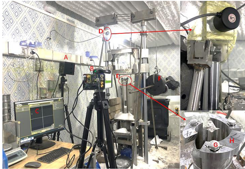
Figure 2. Test stand: A – light source; B – high-speed camera; C – image display computer; D – draw-wire displacement sensor; E – drill bit; F – counterweight block; G – drill bit shoe; and H – cutter.
