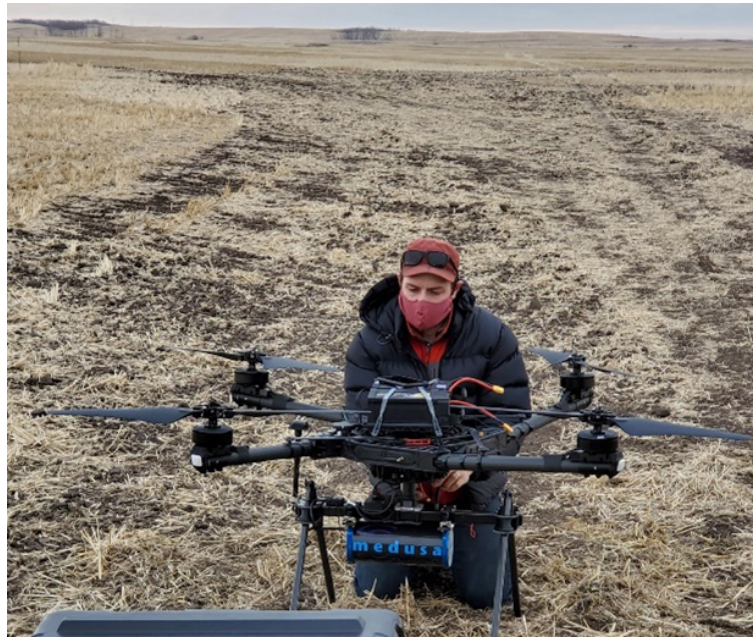
Figure 1. Medusa MS-1000 mounted on a FreeFly AltaX prior to survey 6 November 2020. Photo credit: Anders Hunter.
