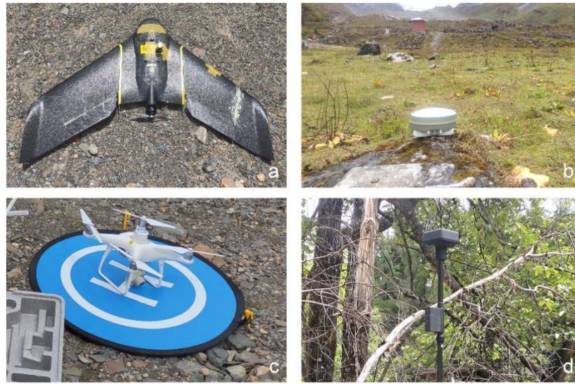
Figure S1. eBee Plus UAV (a), Huaxing A10 GNSS GPS for PPK base station (b), DJI Phantom 4 RTK UAV (c), DJI D-RTK 2 for RTK base station (d).
