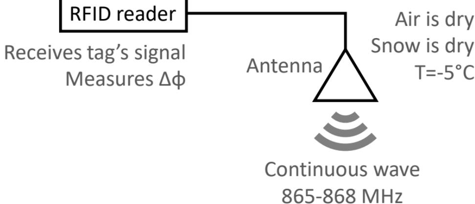
**Adding layers of dry snow to increase the signal phase delay**
