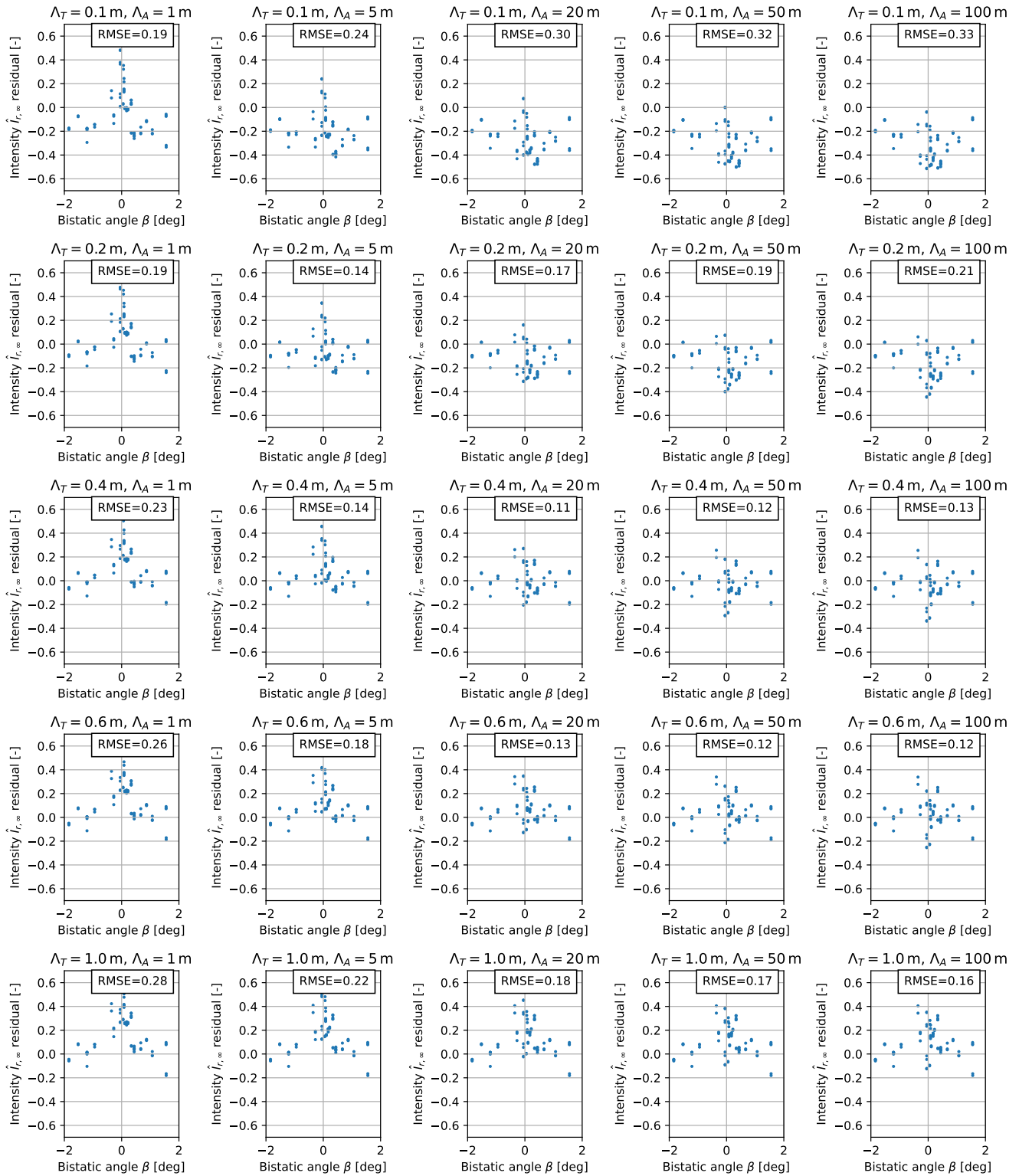
Figure S1. Plots of residuals of winter KAPRI measurements at Davos, Rinerhorn, in the VV polarimetric channel, with varying values of model parameters \Lambda_T (constant along rows) and \Lambda_A (constant along columns). The residual was computed as the difference between observed value of \hat{I}_{r,\infty} and value predicted by the model I_{r,\infty} defined by parameters \Lambda_T, \Lambda_A , at the corresponding bistatic angle \beta .
