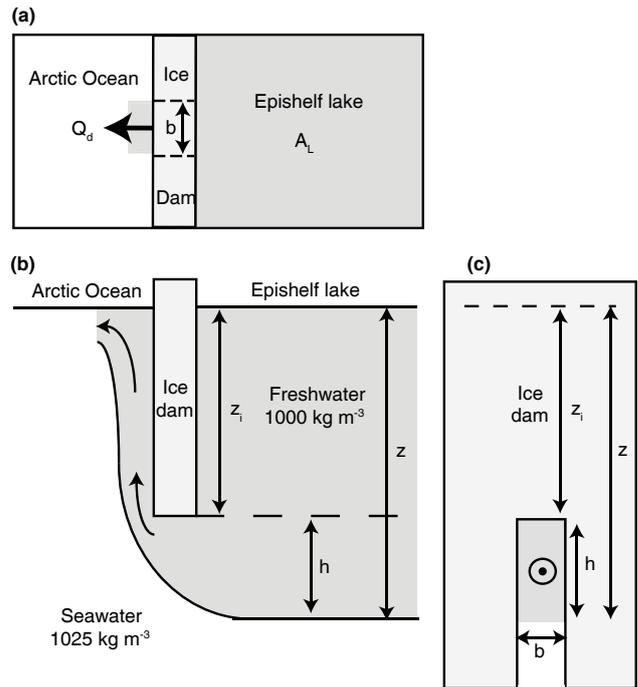
**Figure 10.** Schematic representation of epishelf lake outflow through a basal channel in the ice shelf dam in (a) plan, (b) elevation, and (c) cross-sectional views. The volumetric discharge is modelled using a modified form of the rectangular weir equation (Eq. 7).
