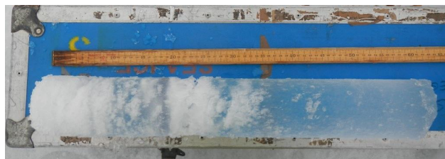
Figure 7. Photo of an ice core extracted from bare ice near the dive hole of the third transect.
