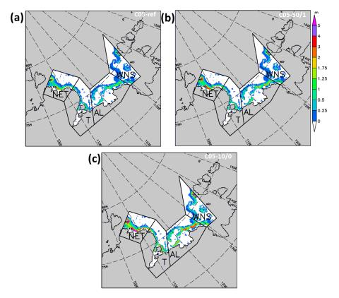
**Figure 11.** Total sea-ice production (m) within the Laptev Sea polynyas in the winter period 2007/2008 simulated by (a) C05-ref (reference), (b) C05-50/1 (realistic), and (c) C05-10/0 (open water).
