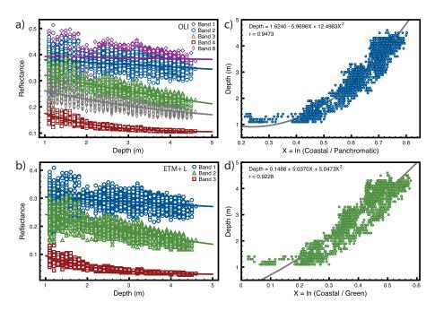
**Figure 2.** Regression plots for in situ measured reflectance spectra used to emulate OLI and ETM+ reflectance and sonar-measured depths, including OLI single band (a), ETM+ low gain single band (b), OLI coastal and panchromatic (c), and OLI coastal and green (d). Statistics for all regressions are reported in Table 1.
